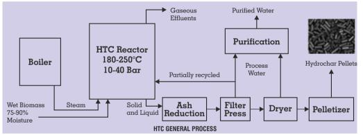
Thermo-chemical reactions are involved in conversion through HTC, which transforms unprocessed waste into a hydro-char bearing a high calorific content and complemented with elevated levels of carbon content. A feedstock with 75%–90% moisture content is considered ideal for this process. HTC comprises three processes, namely, dehydration, decarboxylation and decarbonylation, for which pretreatment or drying of the feedstock waste is not needed.
