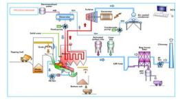
of EfW plant will be configured using simple non-reheat Rankine Cycle concept with
